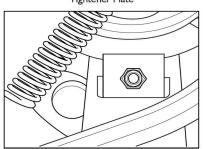
Screw and washer through adapter plate and chair casting.
